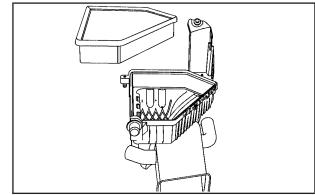
8. Remove the air cleaner element from the air cleaner housing.
